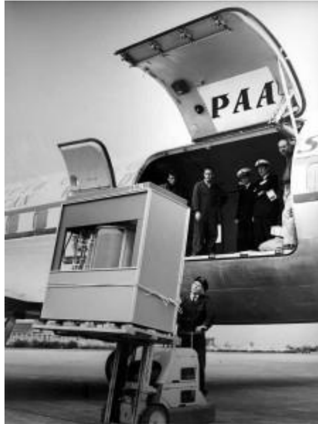
The world's first hard disk drive which held a whopping 3.75MB of data
